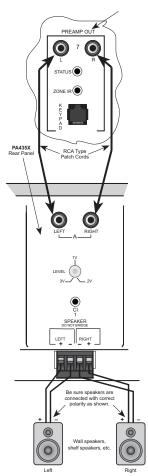
Figure 5 - PA4100X Stereo Mode Connections
